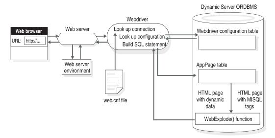
Figure B-2. Web DataBlade Module Architecture
