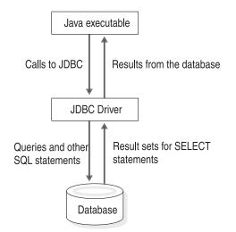
Figure 1-2. Runtime Architecture for Embedded SQLJ Programs
